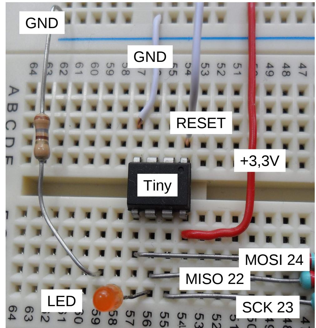
For SPI-communication we need two outputs clock (sck) and data (mosi) and one inut (miso)
